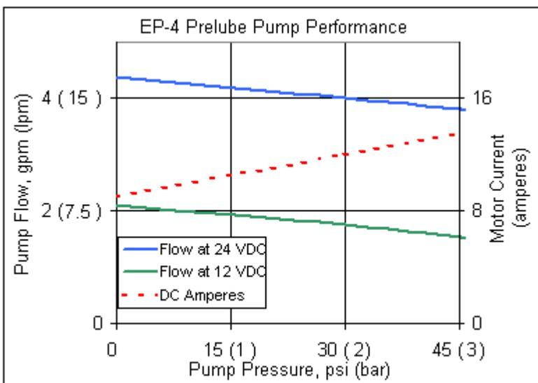
This chart shows the approximate flow and motor load for a given pressure using SAE 40w motor oil. The drop in the flow is caused by a combination of volumetric losses in the pump and the reduction in motor speed as it loads up. Note that at about 35 PSI the current crosses the 7 amp line where duty cycle comes into play. See the following chart.
