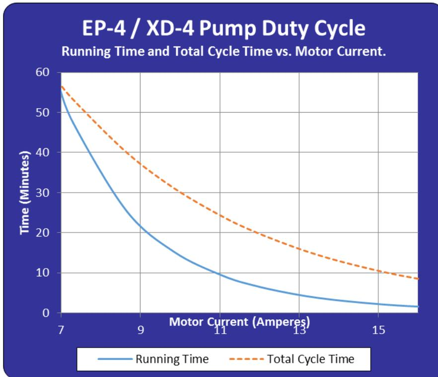
This chart shows the duty cycle for the pumps motor under steady running conditions for a given motor load. It does not take into account a cold motor on the first cycle, which would be somewhat longer. In addition, adding active cooling can substantially improve duty cycle. Running time is the length of time where the pump is running. Total Cycle time is the time from turning on to the time it is next tuned on.
