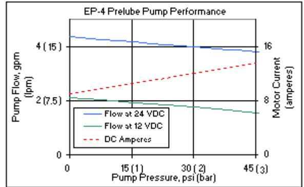
Nominal current draw for the EP-4 pump motor is 15 amps. Motor current varies with pressure. The motor should be fused. See wiring considerations.
