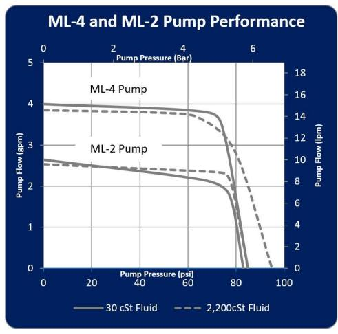
Start by picking a target pressure for the orifice restrictions. Higher pressures need a higher horsepower pump but the diameter of the tubing can be smaller. Lower pressures will require larger diameter tubing but they can use a lower horsepower pump. A good starting pressure might be 30 psi.
